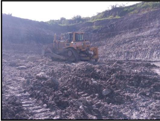
Gambar 1. Proses *Ripping* Batupasir
