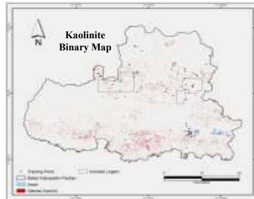
Figure 7. Kaolinit alteration zone after threshhold processing. The rectangular line is concenssion area belong to local companies
